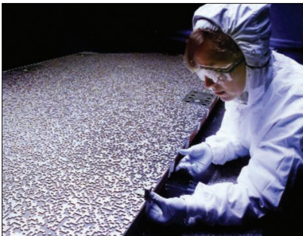
Coded pattern. A lead-tile mask will cast a unique gamma ray shadow on Swift's detector for each burst.
